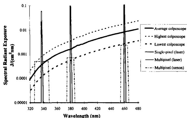
**Figure 2.** Spectral radiant exposure for each spectroscopic system tested and for the lowest, average and highest power colposcopes. Note that the y-axis is a log scale.
