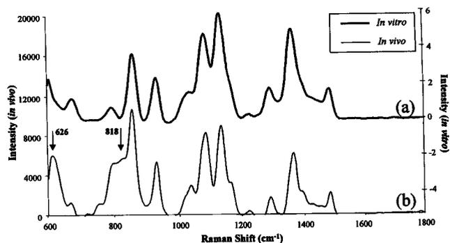
**Figure 3.** The NIR Raman spectra from a dilute solution of glucose (a) measured with the *in vitro* system used in Mahadevan-Jansen *et al.* (9) and (b) measured with the *in vivo* system and probe shown in Fig. 1.
