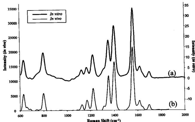
**Figure 2.** The NIR Raman spectra from rhodamine (a) measured with the *in vitro* system used in Mahadevan-Jansen *et al.* (9) and (b) measured with the *in vivo* system and probe shown in Fig. 1.
