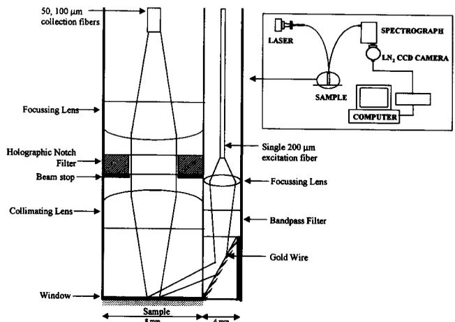
**Figure 1.** Schematic (transverse section) of the probe used for clinical Raman measurements (not to scale) with an insert of the system block diagram.
