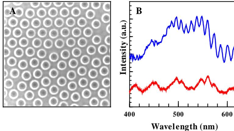
Fig. 4. Density dependence of scattering of 5  $\mu\text{m}$  polystyrene beads in water: (A) a semi-regular monolayer of 5  $\mu\text{m}$  polystyrene beads; (B) depolarization ratio spectra of a water suspension (blue) and of a monolayer of the beads (red).
