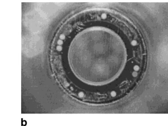
Fig. 1. **a**: Schematic diagram of system used to measure fluorescence excitation emission matrices. **b**: Picture of fiber optic probe tip. The fluorescence collection channel is the inner glass tube that is embedded into a metallic tubing. Reflected white light can be measured with fibers placed along the circumference of the probe.
