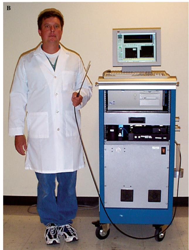
Fig. 3. A) This is a system block diagram or cartoon showing an excitation light source assembly, a fiber-optic delivery system and collection probe, and a polychromator assembly; B) A photograph of the actual device built by our laboratory and being used in the clinic for the pilot trial.
