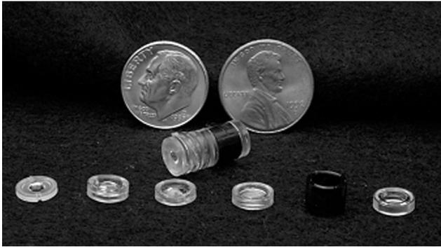
Fig. 3. Injection-molded plastic objective lens assembled and disassembled with U.S. coins.
