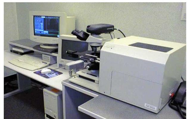
**Fig. 2** Cytosavant<sup>®</sup> is a computer-assisted image analysis system for the quantitative measurement of cytopathology and histopathology. The system consists of an autofocusing microscope, two computers, and an automatic slide loader.
